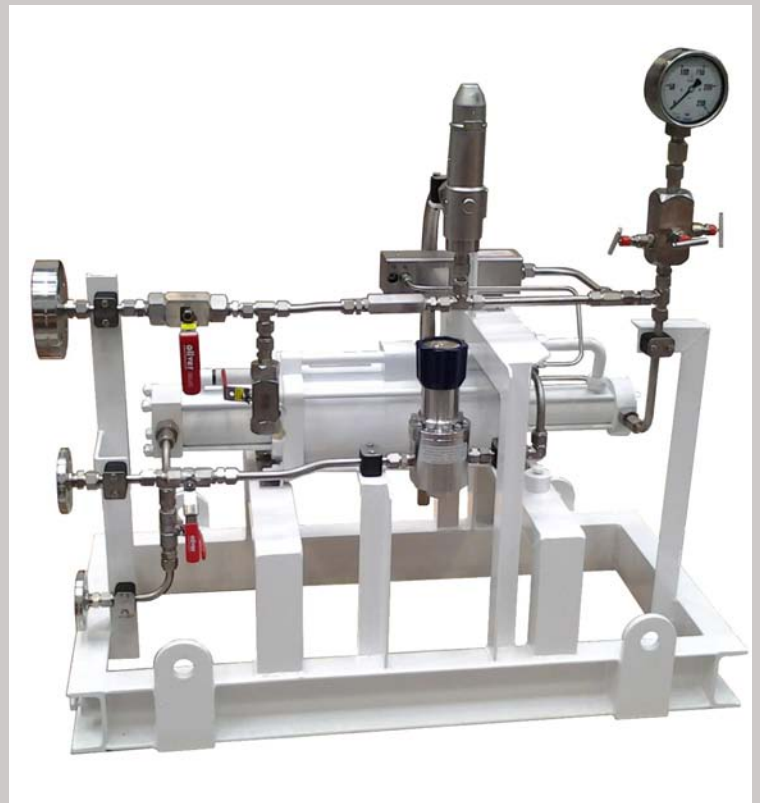
▲ Piston type booster compressor, air driven
