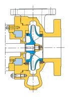
Cooled mechanical seal chamber
